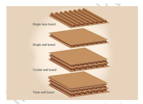
Figure 1: Corrugated box and their contents – Single/Double/Triple wall
